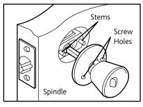
Insert exterior knob with spindle into latch making certain that the stems are positioned correctly through the latch holes. Press flush against the door. Ensure the key section is in the correct position.
