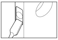
**2.** Chisel a 3mm deep rebate or until the latch face is flush with the door edge.
